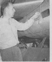
BURTON S. SNOW inspects a camera window opening on a modified U. S. Air Force F 100D.
